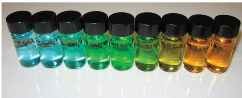
**Figure 1.** Color changes of  $\text{Cu}^{2+}$  solutions ( $0.1 \text{ mol L}^{-1}$ ) in choline chloride/water mixtures with varying water content. The water content decreases from 100 wt % at the left (blue sample) to 27 wt % at the right (yellow sample).
